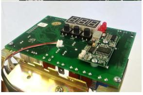
Unplug Strain Gauge from Controller
