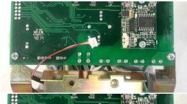
Thread Strain Gauge wire through gap between Controller and bracket
