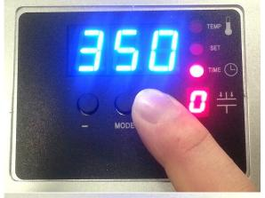
Adjust display reading using (+) and (–) buttons to match temperature strip reading
