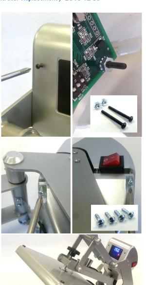
Install 2x #4-40 x 1" Screws and Nuts with Lock Washer using #1 Phillips Screwdriver to secure new Controller to top half of Controller Housing
