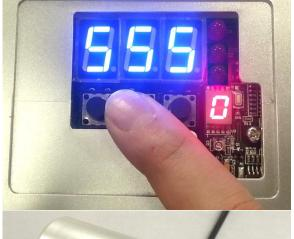
Press and center (MODE) button repeatedly (3 times) until LED indicator lights at right are all off
