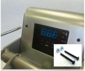
Remove 2x #4-40 x 1" Screws from Controller Housing using #1 Phillips Screwdriver
