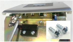
Attach new Controller to top half of Controller Housing by screwing in 2x #6 x ½" Screws using #2 Phillips Screwdriver
