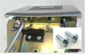
Lift off top half of Controller Housing and remove 2x #6 x ½" Screws from Controller Bracket using #2 Phillips Screwdriver
