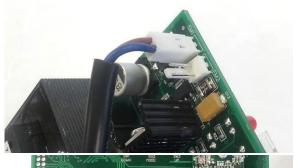
Plug in Electromagnet wire to port EM1 of Controller
