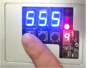
Using caution as the press will open on its own, press and hold (–) button to release electromagnet lock
