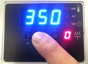
Press center (MODE) button repeatedly (4 times) until LED indicator lights at right are all off
