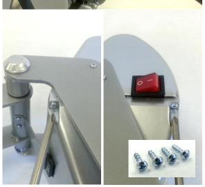
Remove 4x #6 x ½" Screws from control housing using #2 Phillips Screwdriver
