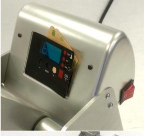
Apply new Overlay to Controller Housing
