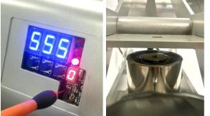
Adjust trim potentiometer as shown using 2mm Precision Flathead Screwdriver until display reads "0"
