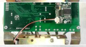
Plug in Strain Gauge to Controller
