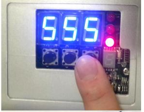
Press (+) button until display flashes "1" indicating pressure reading is below normal range
