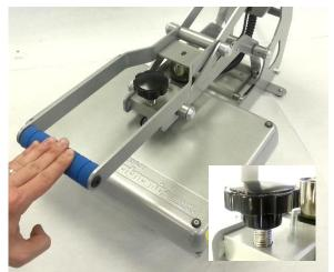
With press OFF, adjust pressure knob to "light pressure" (platen lifts up when locked down in print position)
